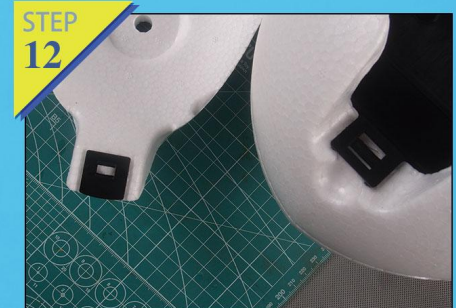
Fig.11-12: Install well the canopy and plastic parts of fuselage by glue.
