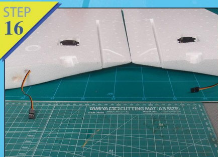
Fig.15-16: Insert servo wire from wing's side slot, and then paste and fix servos.
