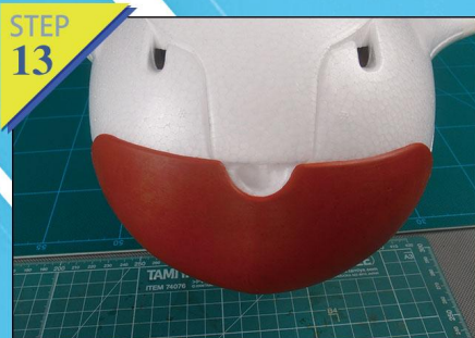
Fig.13-14: Glue its head protection cover, and then insert carbon fiber tube into fuselage. Paste glue between wings and its quick assemble parts and fix them.
