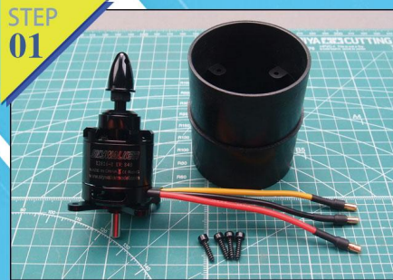
Fig.1-2: Fix motor on the motor mount by 4 screws.
