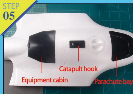
Fig.5-6: Duab glue on the parachute bay, catapult hook, equipment cabin, motor mount and battery plywood.
