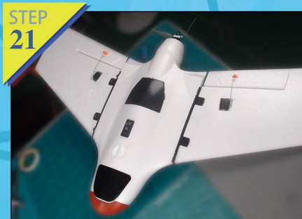
Fig.21-22: Install wings on the fuselage (install them by carbon fiber tube and quick assemble parts).
