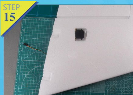
Fig.15-16: Insert servo wire from wing's side slot, and then paste and fix servos.
