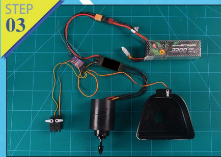
Fig.3-4: Connect ESC and receiver. Return servo to original place and ensure that the motor turns clockwise direction. Fasten plywood of equipment bay by screws which is easy to change receiving equipment.
