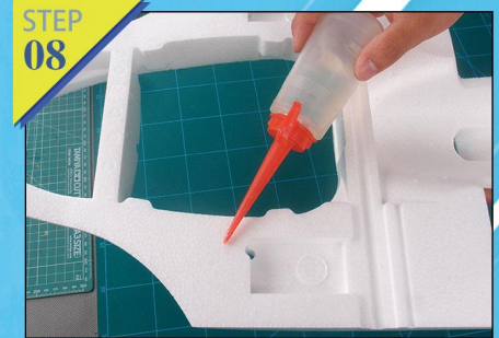
Fig.7-8: Duab glue on both side of fuselage's surface. Air-dry for 2 mins, wait for it until unsticky.
