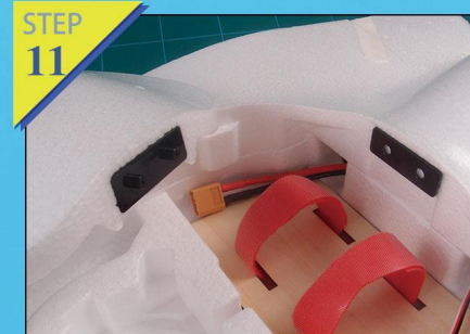
Fig.11-12: Install well the canopy and plastic parts of fuselage by glue.
