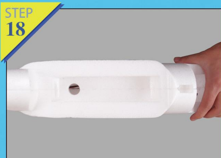
Fig.17-18:Duab glue on the left and right surface of fuselage. Air-dry it for about 3 minutes(according to specific circumstances) and gather up the fuselage.
