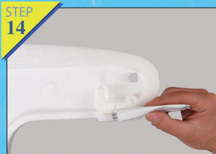
Fig.13-14:Fix the carbon tube into the slot(Attention: keep fuselage straight).
