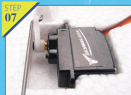
Fig.7-8:Install servo and servo horn. Duab the servo with glue and put it into the slot.
