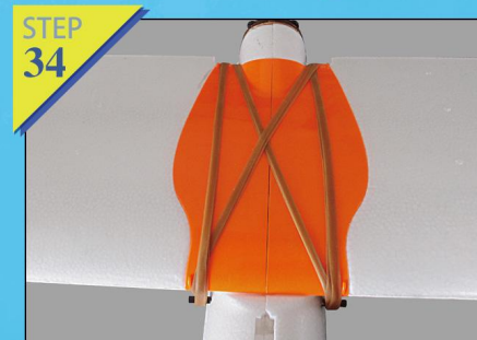
Fig.33-34:Use bungee(2 pieces) to fix wings. Fix it as figure33 and the same way to fix the other side.
