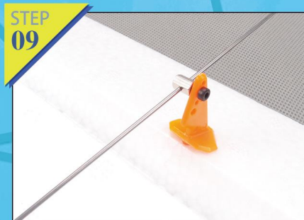
Fig.9-10:Calibrate the servo, and then fasten screws. Cut off the redundant part of pull rod you do not need.Fix the plastic protective cap.The same installation means on the left and right wing.
