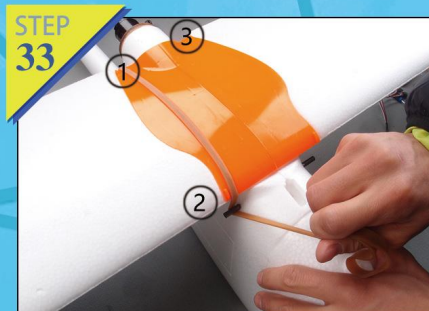
Fig.33-34:Use bungee(2 pieces) to fix wings. Fix it as figure33 and the same way to fix the other side.
