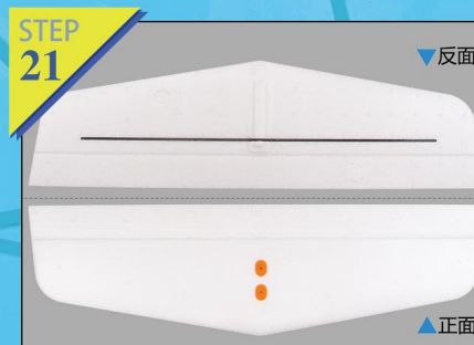
Fig.21-22: Glue reinforcement carbon tube(the same installation of wing carbon bar).Adhere vertical tail plastic part and then fix it on the vertical tail by screws.
