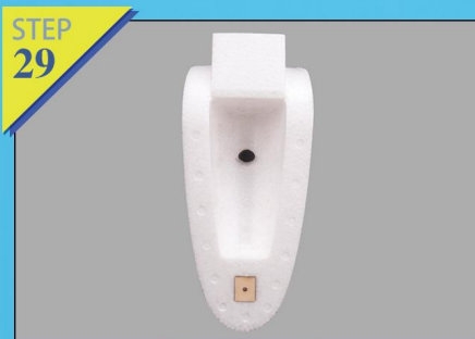
Fig.29-30:Place and paste the small wood piece into slot of its head, afterwards fix it on the fuselage by screws.
