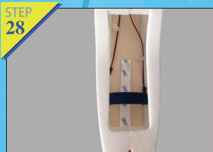
Fig.27-28:Install plywood placed battery. Duab the glue inside cabin and plywood.Air-dry for a while to bond plywood on the cabin.
