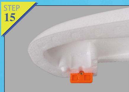
Fig.15-16:Install head's plastic part. Duab glue into the slot(Place the groove surface inside to install head's plastic part).Use the same way to install tail plastic parts.
