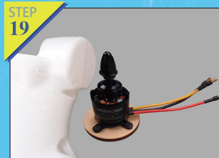
Fig.19-20:Motor base installation(Attention: drill holes on the foam if necessary, do not install propeller before testing to avoid hurting people).
