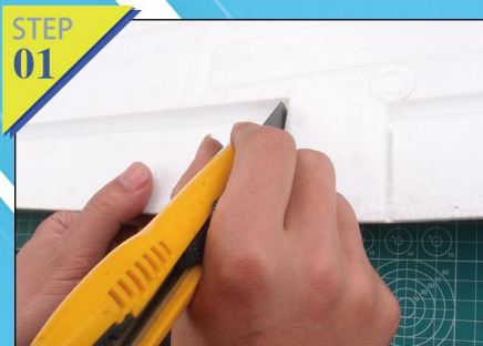
Fig.1-2:Cut the aileron, after that, adhere the cut with fiber tape(the left and right wings are same).
