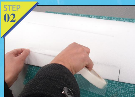
Fig.1-2:Cut the aileron, after that, adhere the cut with fiber tape(the left and right wings are same).
