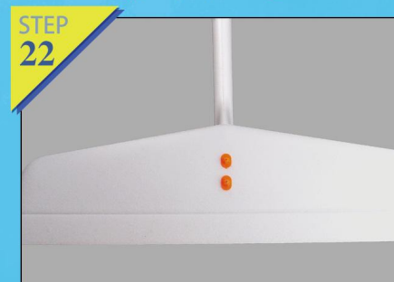
Fig.21-22: Glue reinforcement carbon tube(the same installation of wing carbon bar).Adhere vertical tail plastic part and then fix it on the vertical tail by screws.
